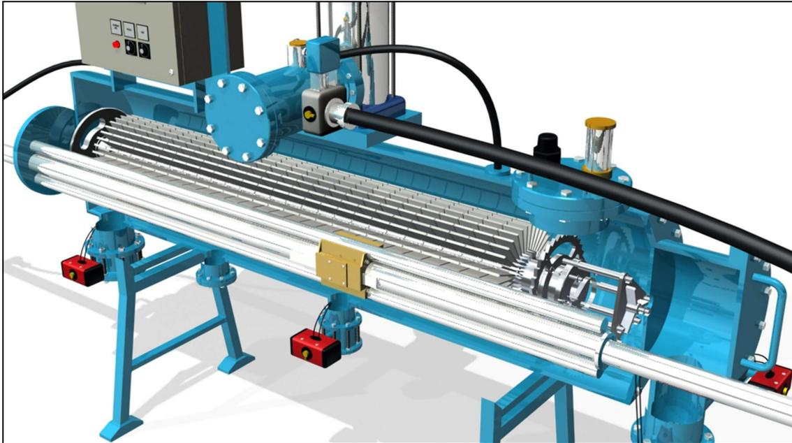
A piston assembly creates an axial movement of the nozzles. A special synchronised indexing mechanism rotates the cassette carousel to a new position when axial movement is completed. When the cassette carousels have completed a full turn, the filter is clean. The drain and backwash valves close, the pump stops, inlet and outlet valves open, and the filter goes back into service.
